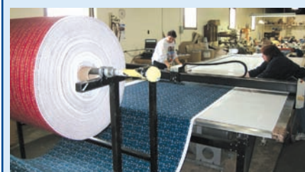
Large rolls of rubber backed fabric are rolled out to over 20 feet and cut into small mat sizes in just five minutes using Red Wing's new automated cutting table.
