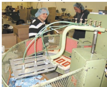
Above, Robert Kurr plans packaging jobs for Apothecary medical products and sends many to ProAct. Below, Apothecary's blister pack machine at ProAct packages pill splitters and other products in Eagan.
