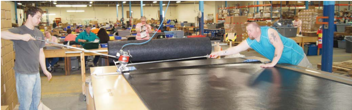
Blake Pommerening, left, and Matt Weisz use a “falcon cutter” to prepare 17- and 20-foot long garage mats for packaging in Red Wing. The 288-by-110 inch table frees up a longtime high-tech cutting table on the work floor for other jobs.
